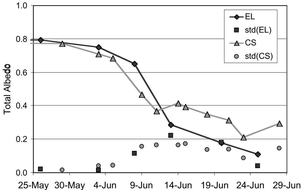
Figure 3: Spectrally integrated albedo averaged over a 200 m observation line on Chukchi Sea and Elson Lagoon during the melting season and standard deviation over each transect.
