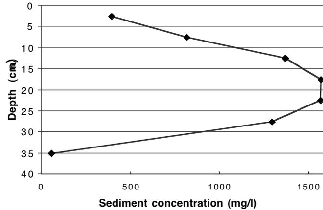
Figure 4: Sediment concentration in the sea ice in Elson Lagoon. The ice below 35 cm did not contain significant loads of sediment, a value of 5 mg/l is assumed.
