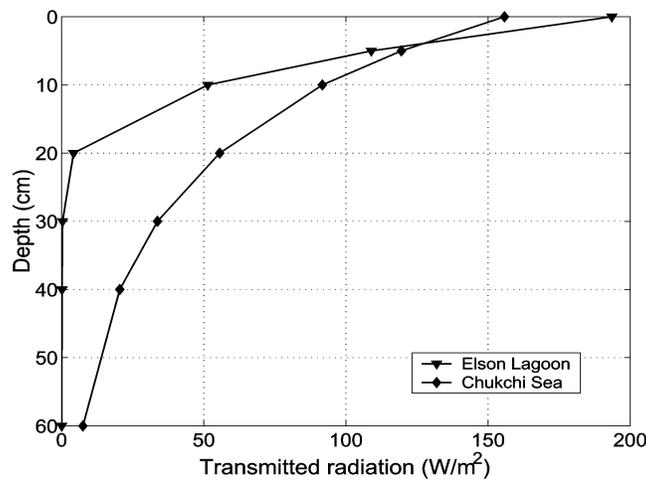
Figure 5: Transmitted radiation as predicted by a radiative transfer model in clean (CS) and sea ice on June 14 with the sediment concentration profile as depicted in Figure 4.
