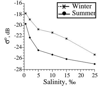
Fig. 4: Backscatter coefficients as a function of surface water salinity from which ice was grown. C-band with incidence angle  $50^\circ$ , air bubble radius 2 mm, brine inclusion radius in deeper layers 0.35 mm (contribution in upper layers neglected due to small volumes).
