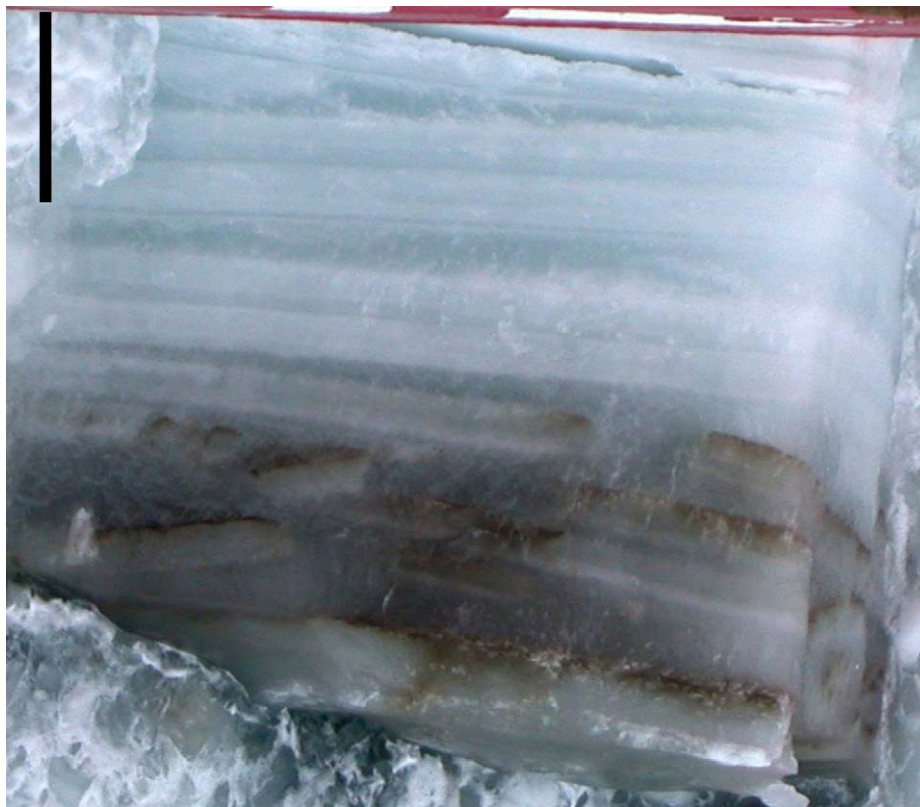
Fig. 5. Stratigraphic cross-section of a level-ice floe turned on its side along icebreaker hull (top is up, scale bar is 0.5 m). Note the multiple rafts stacked on top one another, with the lower rafts associated with sediment particles entrained into the ice cover during growth.
